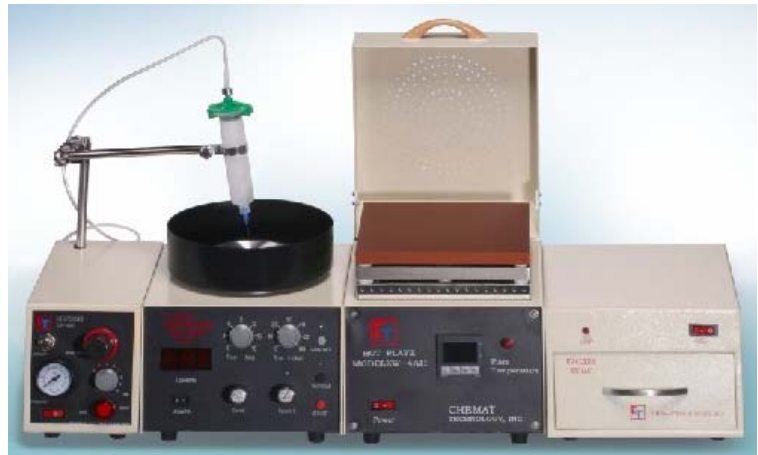
From left to right: dispenser, spin coater, hot plate(350°C), UV curer
